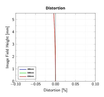
Image Field Height vs. Distortion, from the optical axis to the corner of the image
